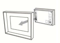
Tighten the screws with the torque between 0.5 N-M and 0.7 N-M to avoid damage to the DOP-105CQ torque: 6.17 lb-inch (0.7 N-M)
