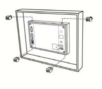
For heat dissipation, please keep a minimum clearance of 60 mm (2.36 inches) and 45 mm (1.77 inches) respectively on the rear and
